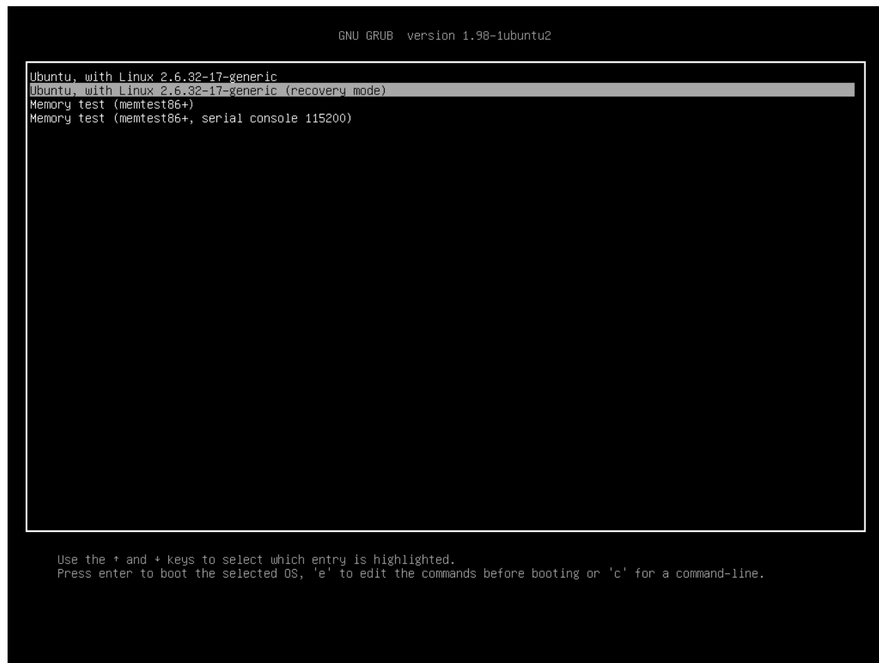
Figure 8.1: This is the grub screen in which you can choose recovery mode.
